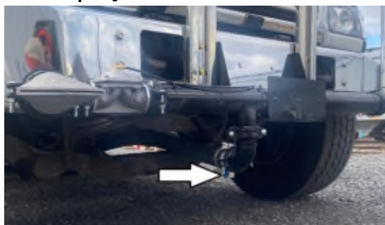
Water Pump Drain Valve
