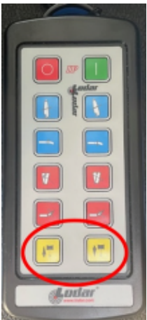
Single Stage Control Box
