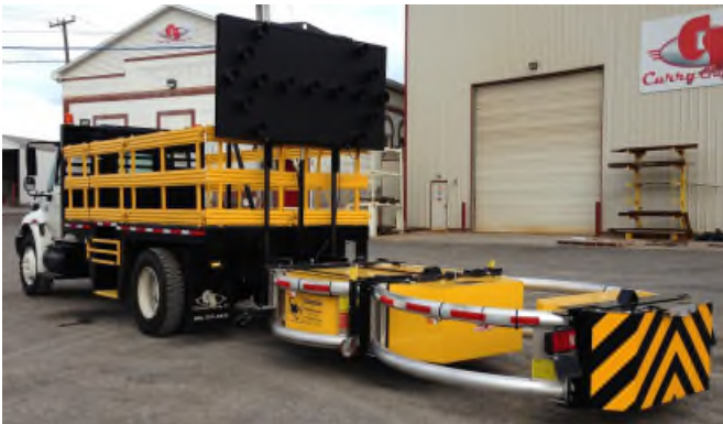
TRUCK WITH ATTENUATOR DEPLOYED
