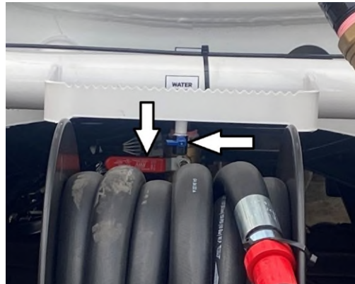
Rear Spray Bar & Tank Drain Valves
