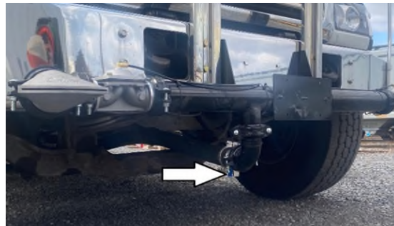
Water Pump Drain Valve
