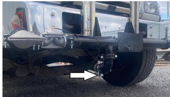
Water Pump Drain Valve
