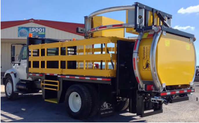
TRUCK WITH ATTENUATOR STOWED
