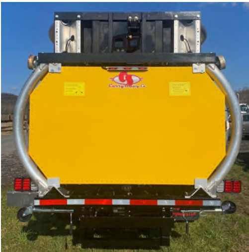
REAR VIEW WITH ATTENUATOR STOWED
