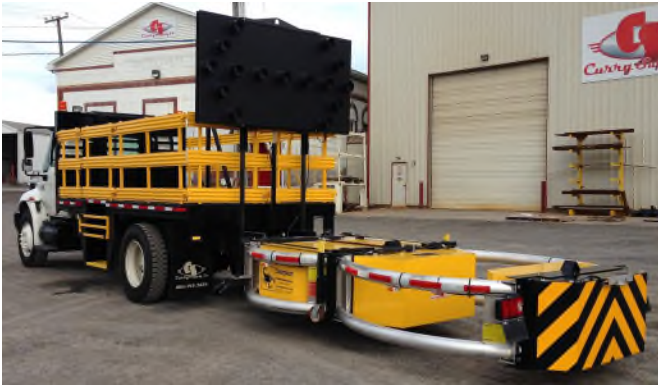
TRUCK WITH ATTENUATOR DEPLOYED
