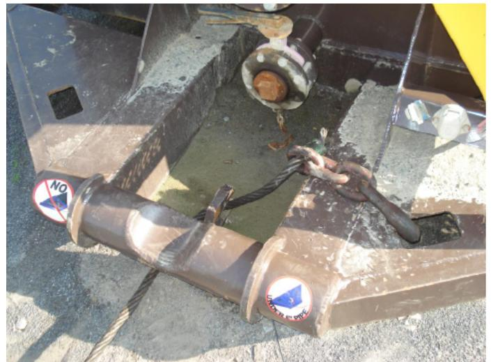
**STEP 4:** Apply the winch brake just enough to keep from creating a bird's nest on the spool. (Not too tight or the brake band will break when pulling forward).
