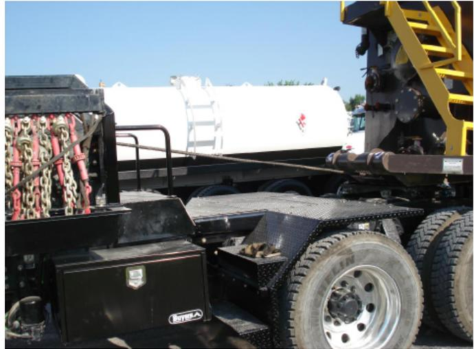
**STEP 5:** Alternate winching the cable out (A) and pulling forward (B) until the tank is over the roller, then stop. (Do not free spool the tank to roller. This may cause damage to the tank or the tractor because the tank will crash to the ground).
