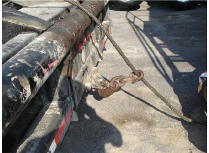
**STEP 8:** Winch the cable in (A) to tighten up the slack (B). (Do not tighten in the cable too much or damage to the suspension and/or the cable may occur).
