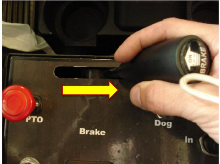
**STEP 9:** Winch the cable in while lightly applying the foot brake on the tractor to keep tension on the cable and then stop before lifting the tank. (Do not winch the cable in loosely).
