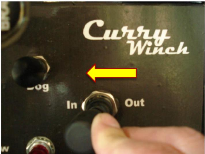
**STEP 10:** Shift the winch into low speed.
