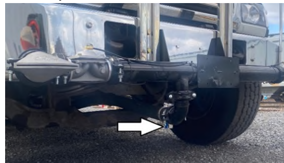
Water Pump Drain Valve
