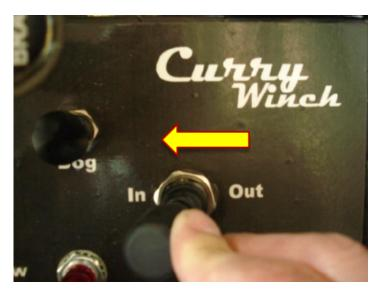
STEP 10: Shift the winch into low speed.
