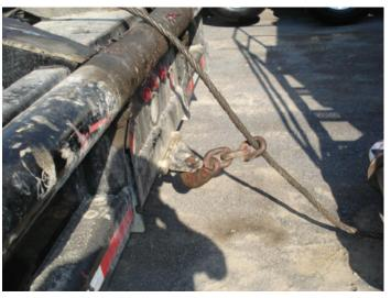
STEP 8: Winch the cable in (A) to tighten up the slack (B). (Do not tighten in the cable too much or damage to the suspension and/or the cable may occur).
