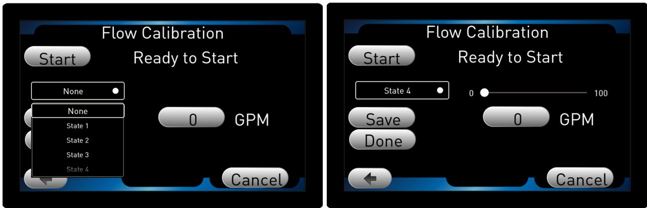
**Figure 50. Multi-Point Flow Calibration Drop-down Menu & Slider**
