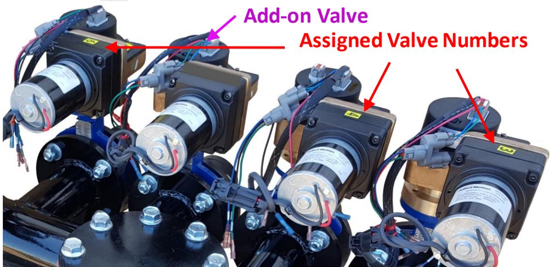
Figure 8. Assigned Valve Numbers
