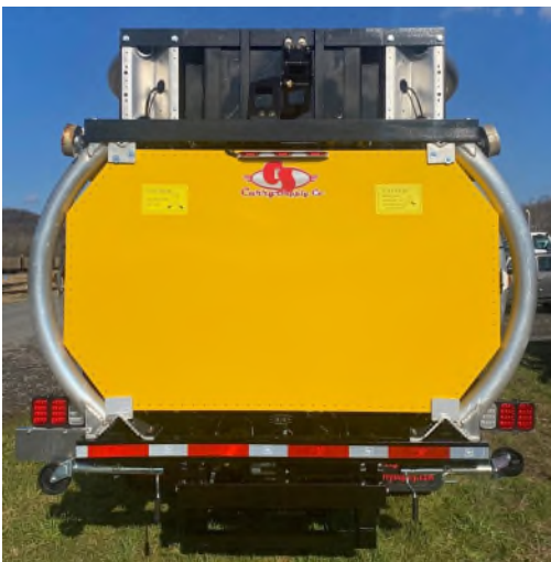
REAR VIEW WITH ATTENUATOR STOWED
