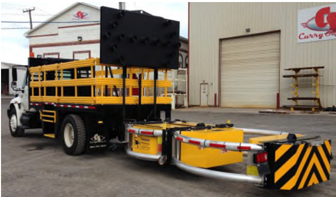
TRUCK WITH ATTENUATOR DEPLOYED
